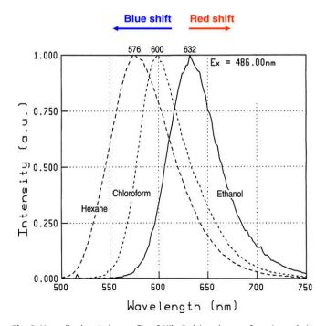
**Fig. 6.** Normalized emission profile of Nile Red in solvents of varying polarity. Dielectric constants were 1.89 for hexane (at 20  $^{\circ}$ C), 4.8 for chloroform (at 20  $^{\circ}$ C) and 24.3 for ethanol (at 25  $^{\circ}$ C). (From Elsey, Jameson, Raleigh & Cooney, 2007).
