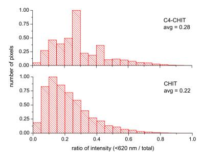
Fig. 8. Ratio of the blue region intensity to the total emission intensity for modified and unmodified chitosan. (For interpretation of color mentioned in this figure, the reader is referred to the web version of this article.)
