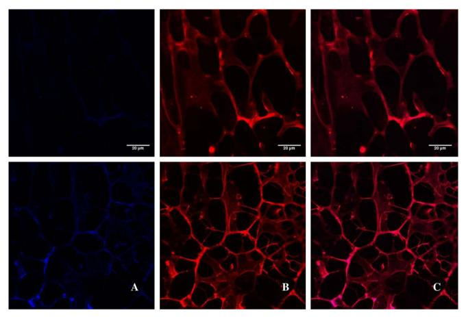
Fig. 7. Laser scanning confocal microscopy images of chitosan scaffolds incorporating Nile Red fluorophore. (For interpretation of color mentioned in this figure the reader is referred to the web version of the article.)
